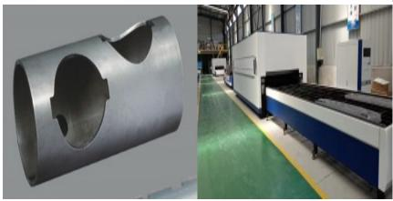
DA-6020 is fiber cutting machine for pipe tube cutting, it manily used to cut round tube, square tube and oval tube, can achieve intersecting curve cutting and arbitrary angle bevel cutting function.
